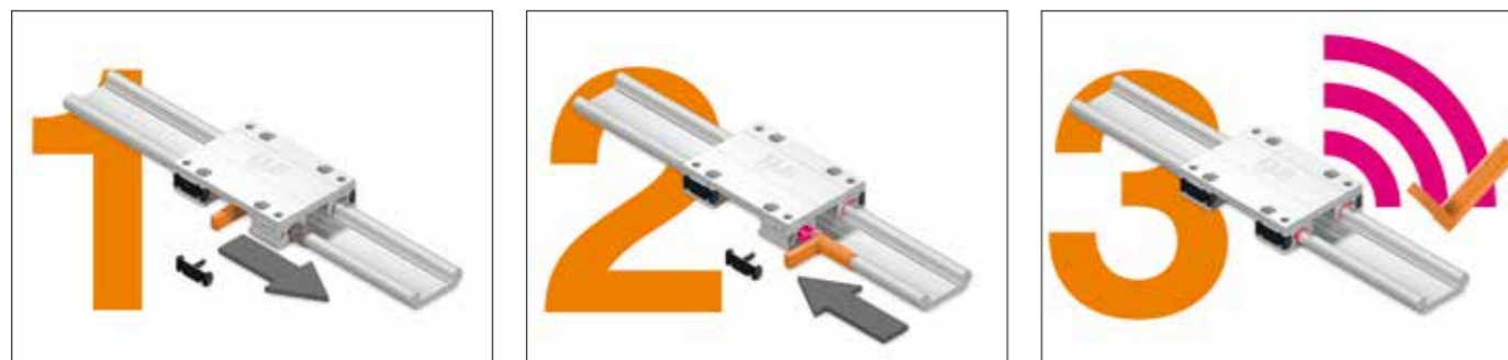
Simple bearing liner replacement.
