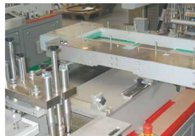
drylin® W guide rails are accredited to cleanroom-standards and therefore used in this blister machine
